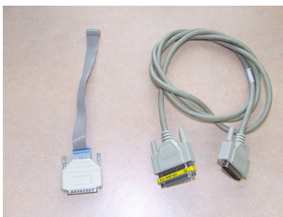
FIG. 1.5 – Photo cordon adaptation JTAG PARALLELE
