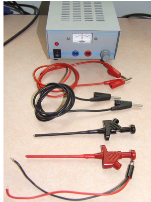
FIG. 1.3 – Photo Alimentation + Cables
