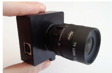
(a) The Dynamic Vision Sensor (DVS).
